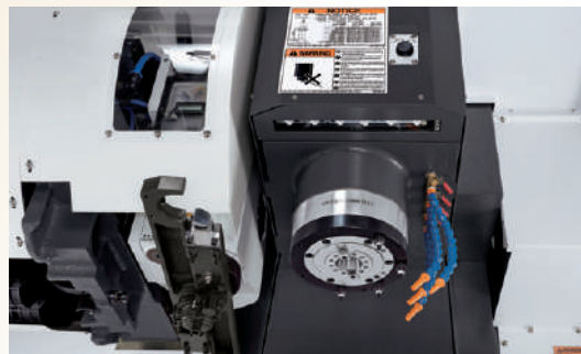
Arm type ATC + Coolant ring + LED lights
