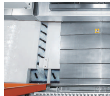
Bottom guarding flush (Vc-F106) + Screw chip removers
