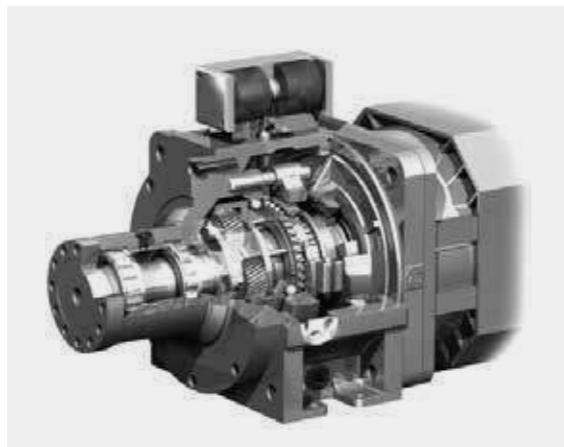
ZF two-speed gearbox has two speed output, which can meet the requirements of low-speed and heavy-cutting of large-diameter workpieces, and also can meet the high speed machining requirements of small-diameter workpieces.
