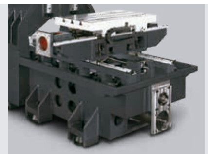
Single Screw Type Chip Auger on Y axis central (EA-600)
