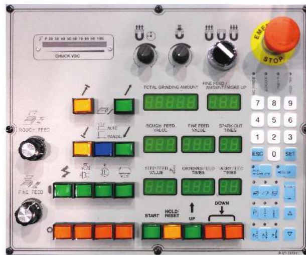
AUTOMATIC DOWNFEED AD5 (NC) CONTROL PANEL (optional)
