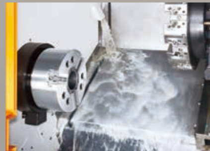
Coolant flush onto covers (Photo with opt. pump Grundfos® MTH 4-4/4)
