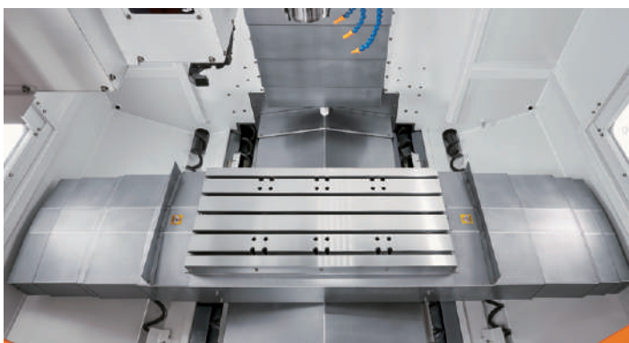
Bottom guarding flush + Screw chip removers
